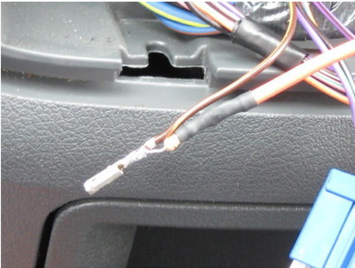
Now solder the rest of the harness to the correct pins. (There's a wiring diagram below to help you out with this.)
