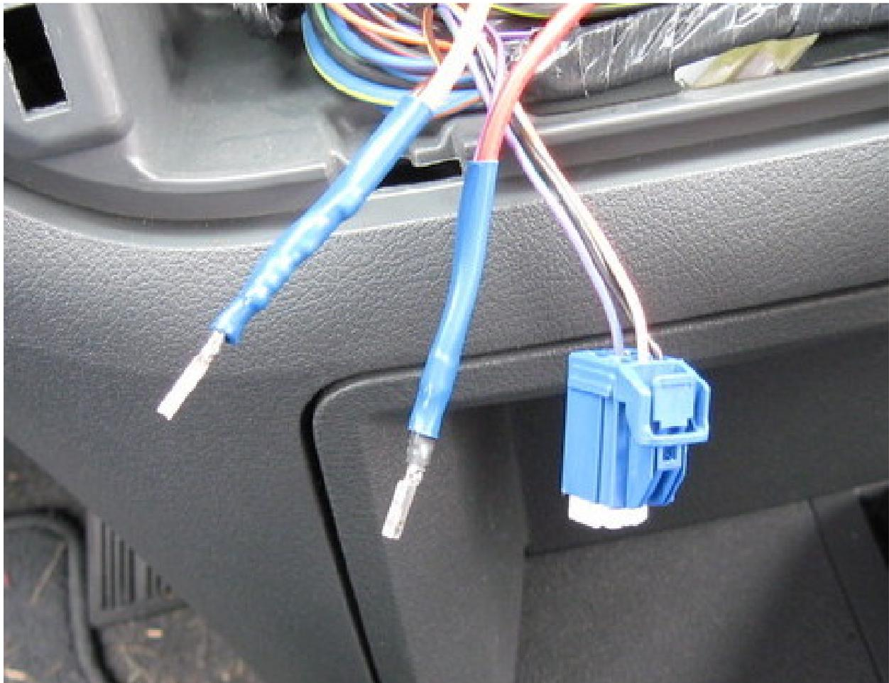
Re-insert all the pins in to their correct locations. Please note that each connector has one pin that is not used, double check the wiring diagram to make sure everything goes back in the right place. Once the pins are in, slide the plastic tabs on the connectors to lock everything.
