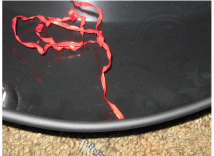
While installing the rubber molding, I discovered that I only had enough to cover 3 1/4 flares. Trying to think outside of the box, I decided that I would attempt to install the front two flares using some 3M double sided tape to see how it held up. I figured I'd see if I liked the tape or the rubber molding better and then I would switch all 4 flares over to my preferred method. So I acquired some tape from the local auto parts store and attached it to the front two flares.
