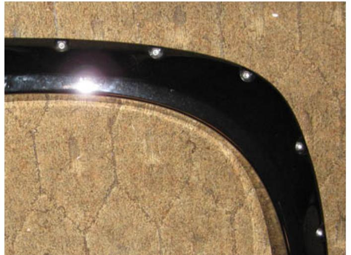
After all the hardware was installed in the flares, it was time to move on to the rubber molding. The rubber molding is to keep the plastic part of the flare from touching the paint of your truck. It's simply a U-shaped rubber strip with some adhesive tape on the inside. Slide it over the edge of the flare from one side to the other, and then cut off the excess. Grab the red plastic cover over the adhesive tape and pull it out. Firmly press on the molding to adhere it to the plastic flare.
