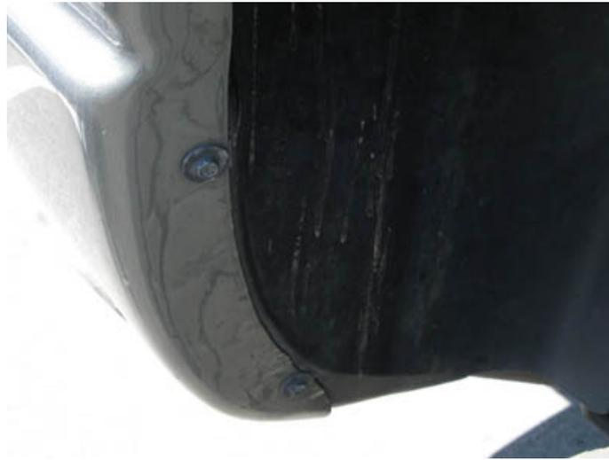
Since the truck doesn't have full inner fender liners installed from the factory, there aren't enough mounting points on the truck to attach the flares. For this reason, the kit includes several clip-on nut plates that you have to install. Install the two smaller nut plates on the forward edge of the fender where the two factory holes are.
