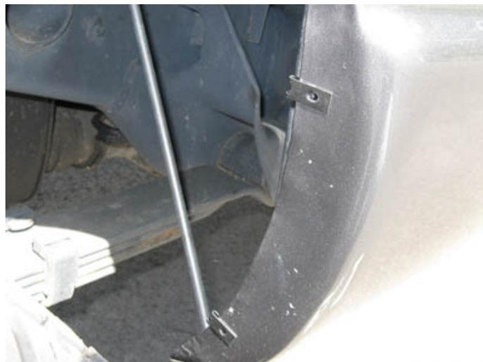
After you install the first two nut plates, hold the flare on the truck and mark the location of the three upper holes and then remove the flare. Apply the supplied tape in the three locations you marked and then slide the three "S" shaped nut plates over the tape. These provide the upper mounting locations without forcing you to drill holes in the truck. The picture below is of a test fit of the nut plate before I put the tape on, then again with the tape.
