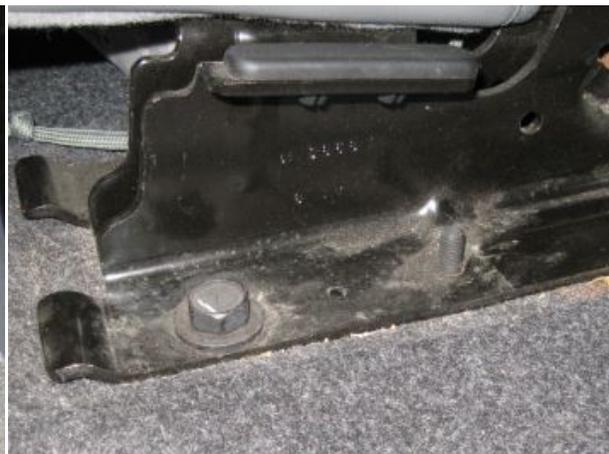
Grab the shelf that matches your side and set it in position over the two studs on the seat bracket. Place the bar on the studs on top of the seat bracket and install the two nuts finger tight.
