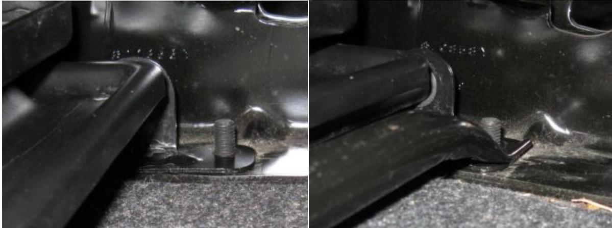
You can now raise the shelf and reinstall the two seat mounting bolts you removed earlier. After the two bolts and two nuts are started, tighten everything down. Repeat this process for the other side.
