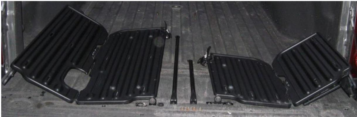
The shelves utilize the forward seat mount bolts and a stud that is pre-welded to the seat bracket. The first thing you need to do is pick a side (driver or passenger, it doesn't matter) and remove the front two seat mount bolts. They have thread locker on them from the factory and will be tight.
